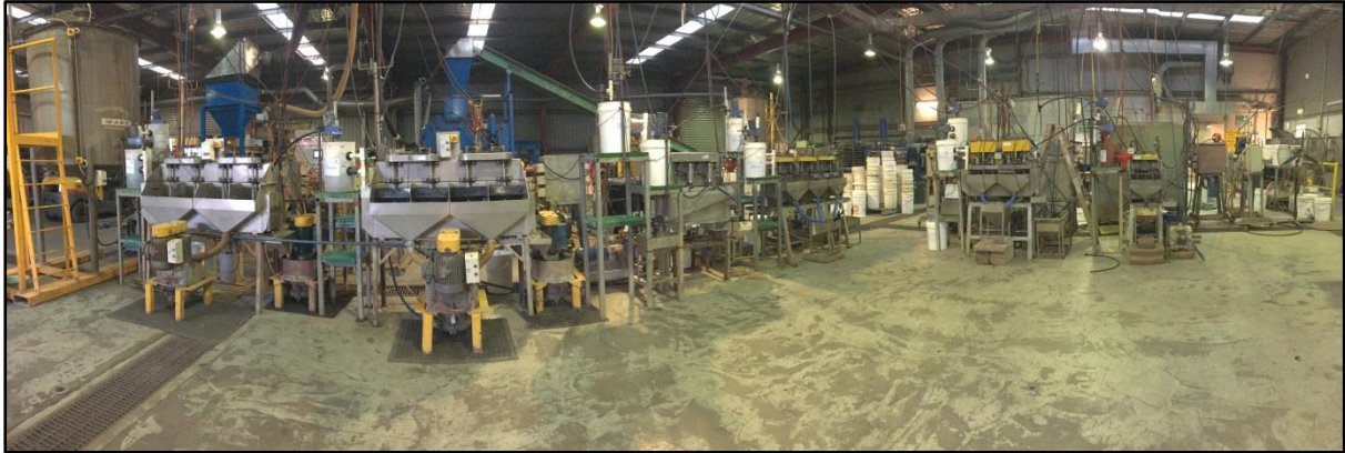
Figure 1 Flotation Pilot Plant Operation at ALS Metallurgy, Perth
