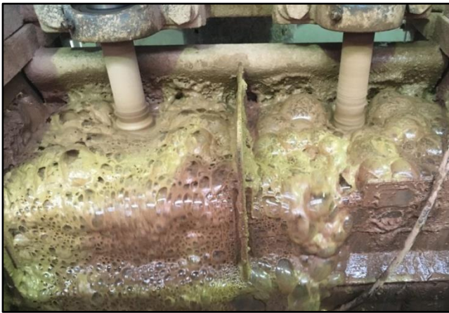
Figure 2: Close-up of Monazite Flotation
