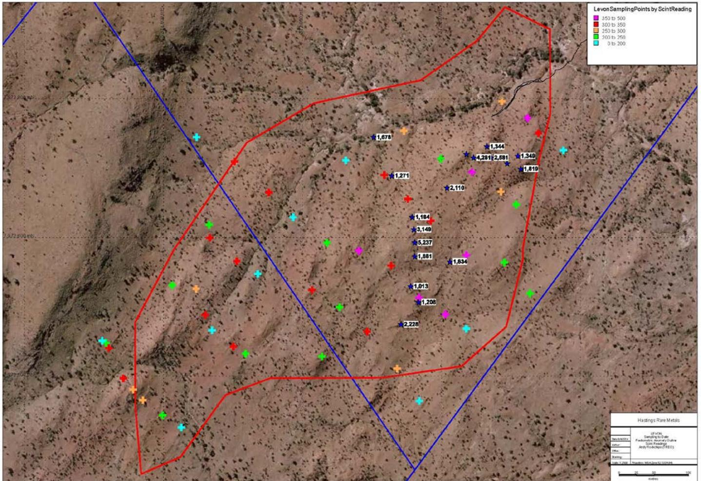
Figure 1 – Levon Prospect. Scintillometer readings April 2014, with previous rock chip sample assays and airborne radiometric (thorium) anomaly
