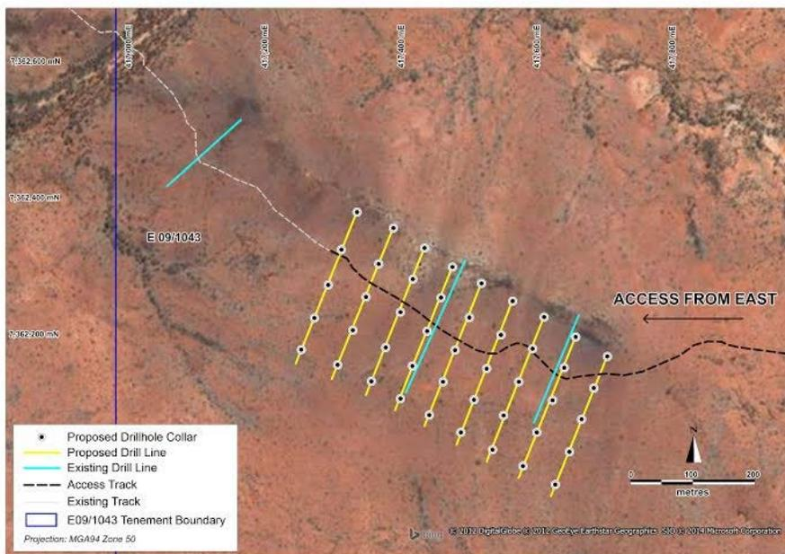
Figure 3 – Aerial view of proposed drill sections
